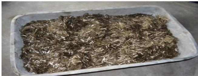
Fig -3 Basalt fibres
