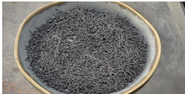
Fig -1 Steel fibres
