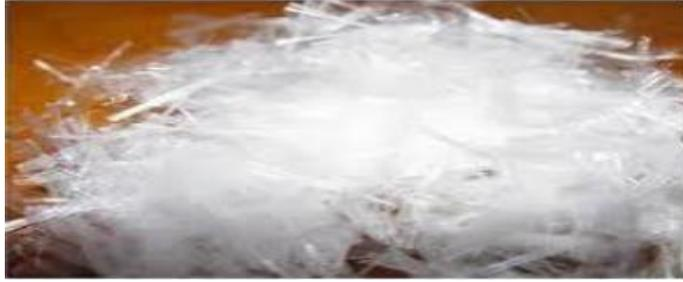
Fig -2 Polypropylene fibres (*Madhavi et al. 2014*)
